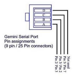
A graphical representation of the Gemini Serial socket is pictured left (i.e. Pin D is closest to the top of the Gemini main Panel)
